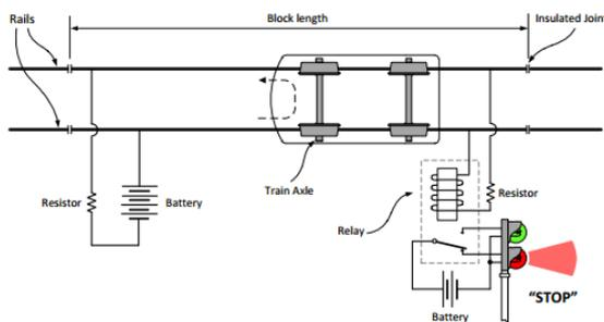
Figure 1: Track Circuit
