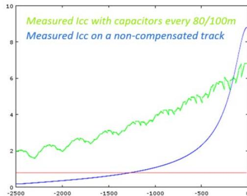
Figure 2: Shunted Current diagram with and without compensating capacitors
